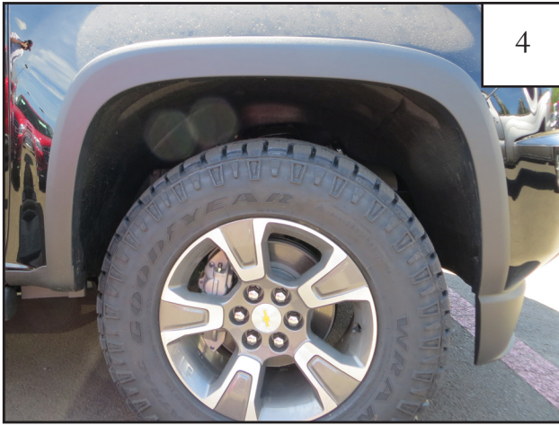
Fitment Note: If factory flares are installed, remove before starting installation. Factory fasteners require a T-15 torx bit.
