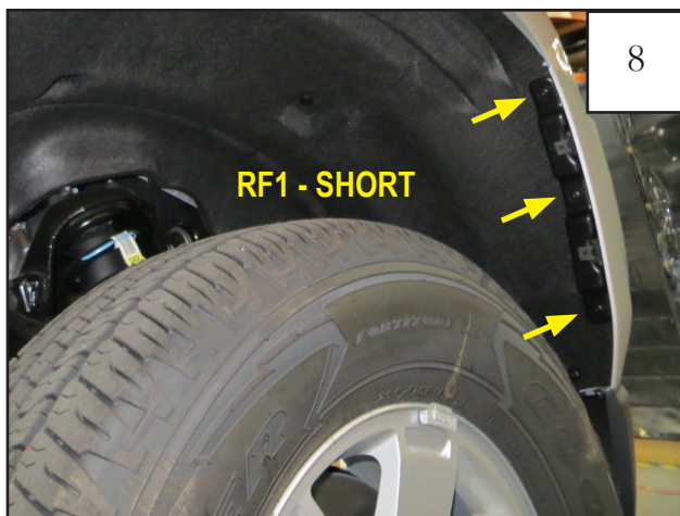
Install the short mounting bracket (RF1) into front of wheel well, using three factory fasteners and a T-15 torx bit. Tighten screws.
